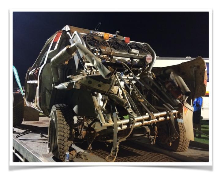
THIS IS A GREAT EXAMPLE OF HOW A WELL-BUILT ROLL CAGE - AND ALL OF THE ITEMS MENTIONED IN THIS SECTION - CAN SAVE YOUR LIFE. THIS VEHICLE HAD A STEERING FAILURE AT HIGH SPEED, ROLLED END-FOR-END SEVERAL TIMES THEN BARREL-ROLLED. BOTH OCCUPANTS SURVIVED WITH NON-LIFE THREATENING INJURIES.
